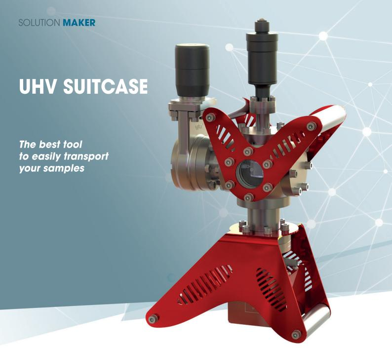
Our ultra compact UHV suitcase is designed to carry up to 5 Omicron type sample plates\* under ultra high vacuum (UHV) conditions (P  $\sim$  10-10 mbar). The original pumping solution based on a Non Evaporable Getter (NEG) allows to keep UHV conditions even without powering and makes easy long trip transports and aircraft travelling.
