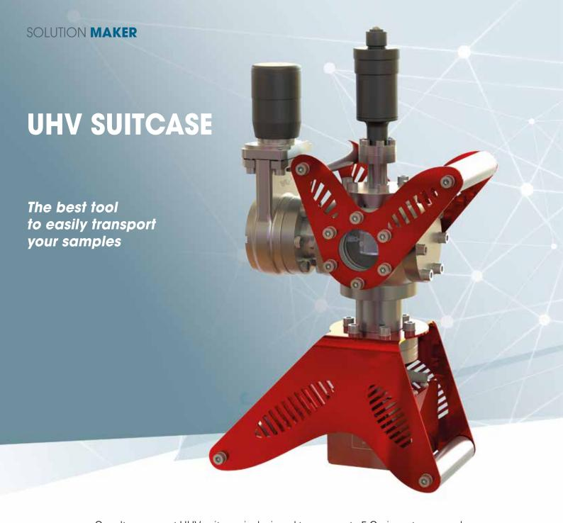
Our ultra compact UHV suitcase is designed to carry up to 5 Omicron type sample plates\* under ultra high vacuum (UHV) conditions (P ~ 10-10 mbar). The original pumping solution based on a Non Evaporable Getter (NEG) allows to keep UHV conditions even without powering and makes easy long trip transports and aircraft travelling.
